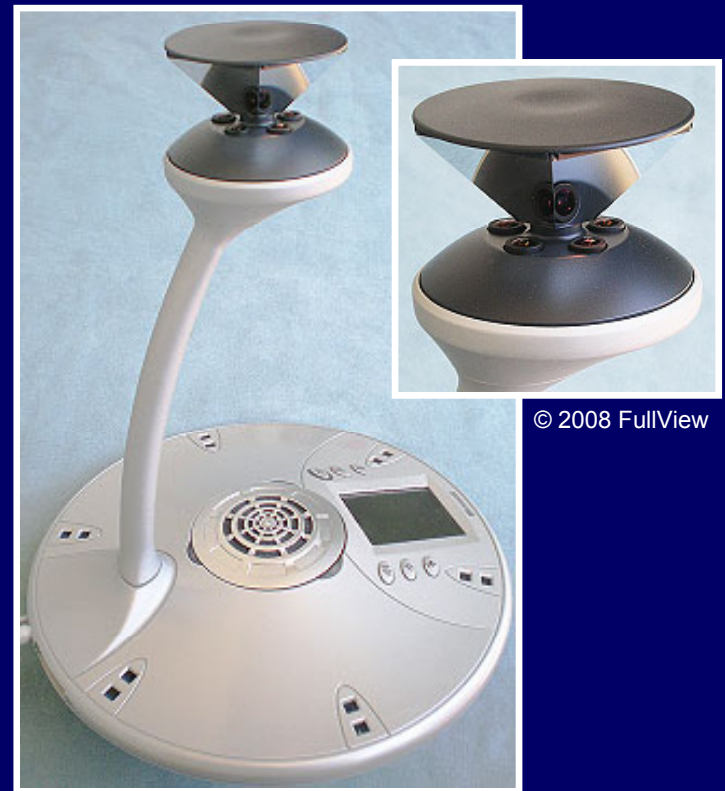
Cameras Looking Out Off Mirrors, After FullView License
